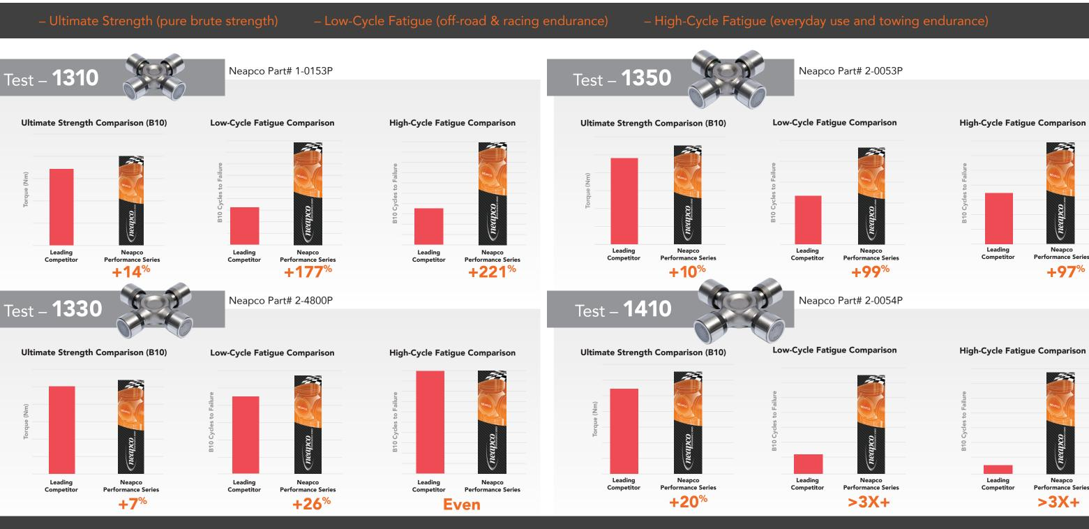
Neapco Performance Series Universal Joints are Made in the U.S.A and are immediately available in the following series and conversions: 1310=Part# 1-0153P; 1330=Part# 2-4800P; 1350=Part#2-0053P; 1410=Part# 2-0054; 3R=Part# 2-3011P; 7290=Part# 2-1175P; 1330/3R=Part# 2-1569P; 1330/7290=Part# 2-0355P; P55-55-675=Part# 2-4900P COMING SOON 1480 and 1550 Series
