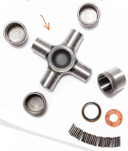
Leading Competitor U-Joint after rigorous head-to-head testing
