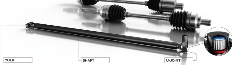
CNC machined as an exact fit to OE Hot forged high carbon steel for optimal strength and durability DOM (drawn over mandrel) tube provides more exact ID and OD values
